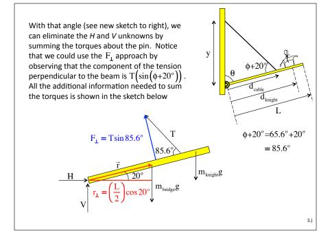
We need to know the angle between the cable and the beam. This is going to require some trickery. Consider the sketch shown below:
